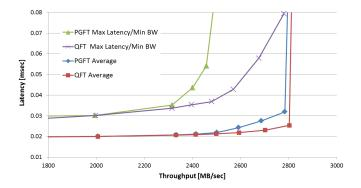
Fig. 3. Simulation results showing latency vs. throughput curves, parameterized by offered load, for PGFT and QFT. The simulated cluster has 4536 hosts and runs 12 concurrent jobs. Job are placed in fragments of contiguous-placement of size distributed as Normal(36,10).
