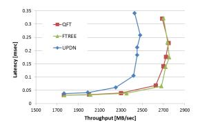
Fig. 9. Latency-versus-Throughput curve for multiple jobs placed randomly on a QFT of 4536 hosts with 56Gbps InfiniBand links. The routing algorithms updn+scatter, ftree and qft show saturation at 2480MB/s, 2740MB/s and 2740MB/s respectively.
