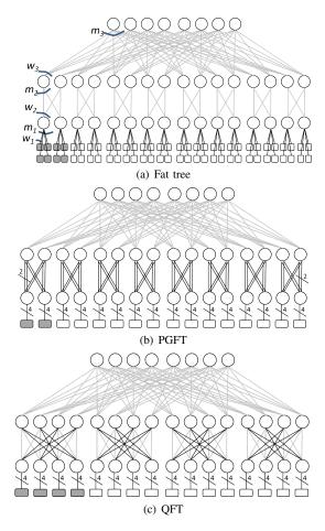
Fig. 1. Fat tree, PGFT and QFT topologies with 64 hosts and 40 switches of 8 ports. (a) A non-maximal Fat tree, thus leaving 2 unused ports in middle and lower level switches (b) PGFT utilizing the free ports by adding parallel links between the low and middle level switches; (c) QFT where the leaf switches connect the unused ports to different switches. As a result, the size of host groups that are within a 3-switch distance is doubled (as denoted by the shadowed hosts).
