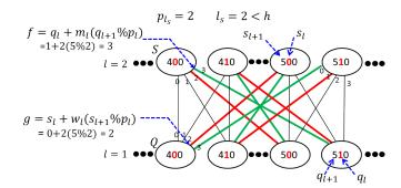
Fig. 6. Example of QFT connection rule, given a subset of a QFT in levels 1 and 2(< h). The extra cross-connections that do not appear in the fat tree are drawn using wider lines. For instance, there are  $p_2=2$  cross-connections from level-2 switch to level-1 switches, in addition to the 2 regular connections.
