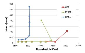
Fig. 8. Latency-versus-Throughput curve for a single job executing random shift permutations on a QFT of 4536 hosts with 56Gbps InfiniBand links. The routing algorithms updn + scatter, ftree and qft show saturation at 2620MB/s, 4400MB/s, and the full link bandwidth respectively.
