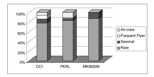
Figure 3-2: Distribution of different trace types in different applications.
