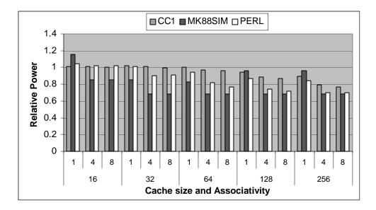
Figure 4.5: Relative power consumption of a filtered T\$ vs I\$
