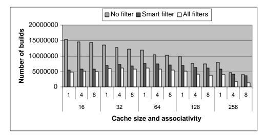
Figure 4.2: number of builds for various trace cahce configurations (CC1)
