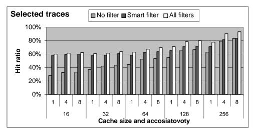
Figure 4-1 trace cache hit rate using 3 filtering options (CC1)
