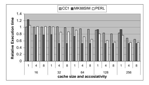
Figure 4-4: Relative execution time of a filtered T\$ vs. I\$
