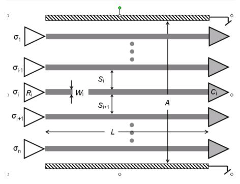
Fig. 3 A fundamental model of interconnecting bus comprising parallel wires laid on the same layer between two shielding wires
