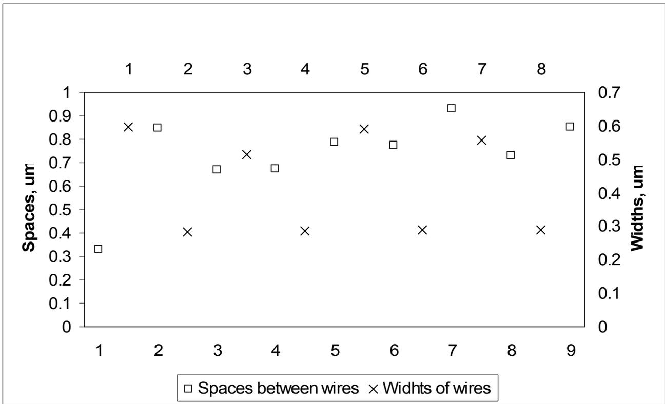
Figure 9: Non uniform bus total sum of delays optimization
