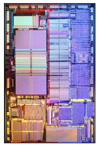
Figure 2: Intel486 Processor -- counter-clockwise from top-left: memory interface, 8k unified cache, floating point unit. At the bottom right is the decode logic, microcode ROM at bottom all mostly hand-craft, then going up split into data-path on left (hand-craft) and control on right (all synthesis with a small hand-craft section in middle of die), crossing control signals handled by full-chip assembly. Photo courtesy of Intel Corporation.
