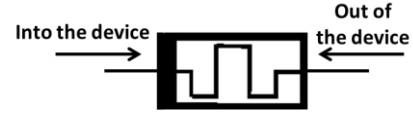
Figure 1. Memristive device symbol. The thick black line on the left side of the device represents the polarity of the device. If the current flows into the device, the resistance of the device decreases. If the current flows out of the device, the resistance increases.
