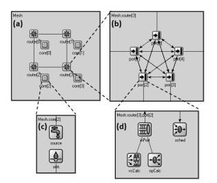
Figure 1. 2x2 mesh NoC: (a) a complete mesh built from routers and cores; (b) a hierarchical router of 5 ports; (c) a core structure; (d) a single port structure.
