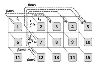
Figure 7. Synthetic example of NoC with non-uniform numbers of VCs and non-uniform capacities of links (Unless noted links are 16Gbps and have sufficient number of VCs).  $C_{l_2} = 10 \ Gbps; C_{l_{12}} = 12Gbps; V_{l_7} = 1.$
