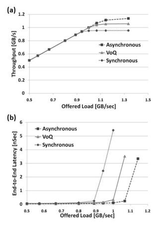
Figure 5. Uniform traffic pattern. (a) Average throughput versus offered load ; (b) Average end-to-end latency versus offered load
