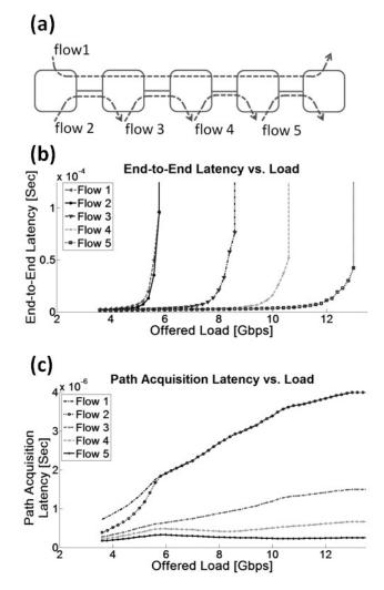
Figure 6. (a) Synthetic Example for Non-Uniform Traffic ; (b) End-to-end latency versus offered load per flow ; (c) Path acquisition Latency versus offered load per flow
