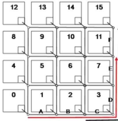
Fig. 2. Flows from core 0 to 11 and 2 to 15 using common links C, D and E but GAU is able to avoid contention by controlling the exact time each packet is injected into the network
